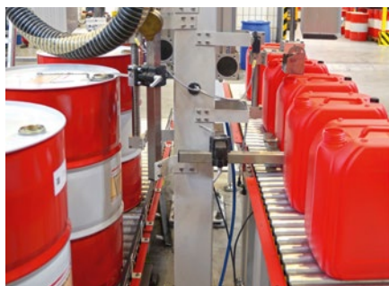
Flexible filling of cans and drums
